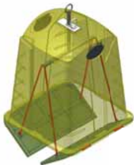
Emptying mechanism - paper, plastics
